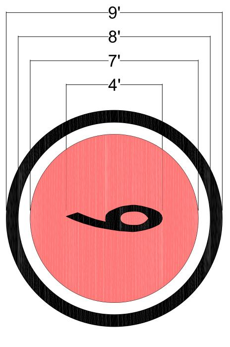
AirMark preformed thermoplastic markings meet the AC 150/5370-10E Item P-620 2.2e and 3.6 Taxiway and Runway Painting Specification for use on Taxiways, Aprons, Ramps and Gates.
