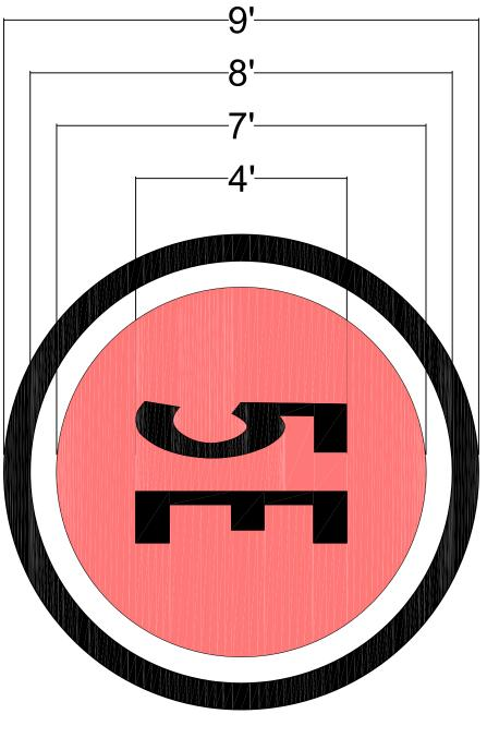
Flint Trading, Inc. has prepared these submittal drawing(s) based upon the purchaser's direction specifically for the manufacturing of Airmark® pavement markings. It is the responsibility of the purchaser to verify and approve the colors/dimensions shown in the respective drawing(s) and, if required, to comply with AC 150/5340-1K. Any change in the marking design after written approval of drawings has been received by Flint Trading may result in
